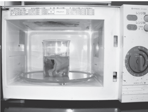
Figure 3. Microwave irradiation of the specimen, and fixation for 3 minutes at around 65°C.
